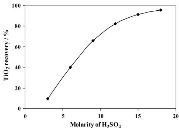
Fig. 4. Effect of sulfuric acid concentration on percentage recovery of TiO<sub>2</sub> (sample not pulverized, no ashing, 0.4 g digestion catalyst added, 4 min digestion, 2 ml of 18.0 M H<sub>2</sub>SO<sub>4</sub>).
