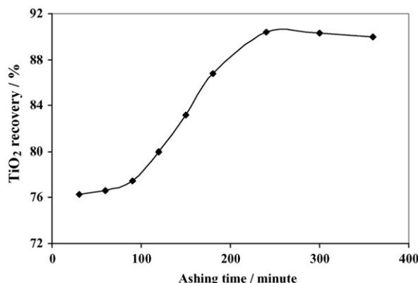
Fig. 2. Effect of ashing time on the percentage recovery of TiO<sub>2</sub> (sample not pulverized, no digestion catalyst added, 4 min digestion, 1 ml of 18.0 M H<sub>2</sub>SO<sub>4</sub>).
