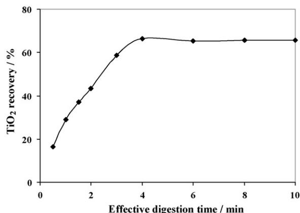
Fig. 1. Effect of effective digestion time on the percentage recovery of TiO<sub>2</sub> (sample not pulverized, no ashing, no digestion catalyst added, 1 ml of 18.0 M H<sub>2</sub>SO<sub>4</sub>).
