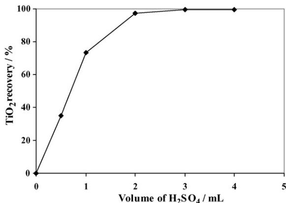
Fig. 3. Effect of sulfuric acid volume (18.0 M) on percentage recovery of TiO<sub>2</sub> (sample pulverized, no ashing, 0.4 g digestion catalyst added, 4 min digestion).
