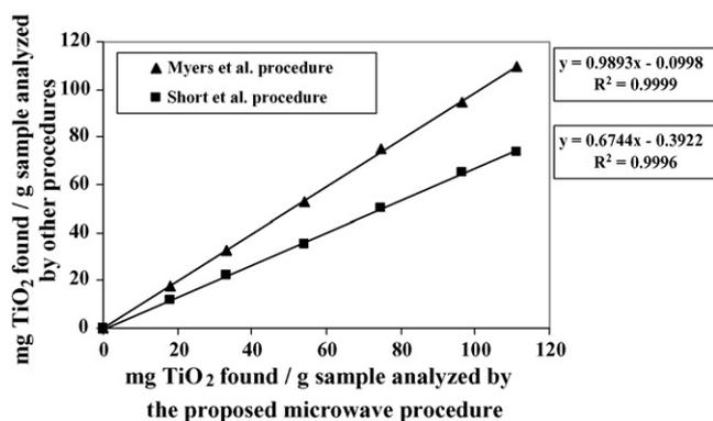
Fig. 6. Relationships between the found TiO<sub>2</sub> using the proposed microwave procedure against the found TiO<sub>2</sub> using Myers et al.'s procedure and Short et al.'s procedure.
