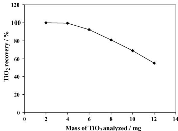
Fig. 5. Effect of mass of TiO<sub>2</sub> analyzed (sample mass) on percentage recovery of TiO<sub>2</sub> (sample pulverized, no ashing, 0.4 g digestion catalyst added, 3.00 ml of 18 M H<sub>2</sub>SO<sub>4</sub>, 4 min digestion).
