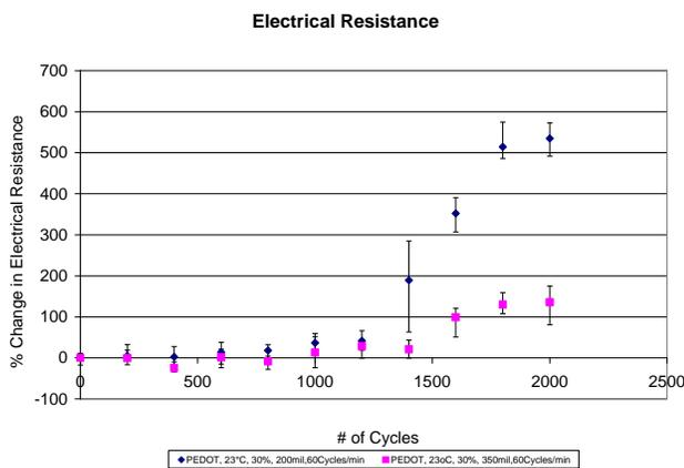
Fig. 6: Effect of bending diameter on the percent change in electrical resistance, the experiments were conducted on an 8 mm-wide sample at a temperature of 23°C, a relative humidity of 30%, and a bending frequency of about 100 cycles/minutes
