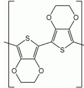
Fig. 1: Chemical structure of Poly (3, 4-ethylenedioxythiophene)
