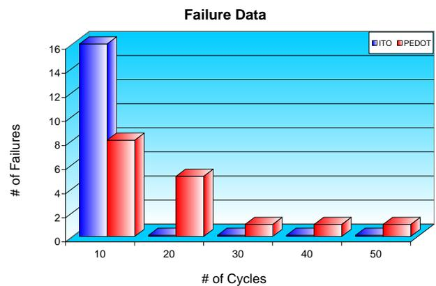
Fig. 7. Conductive failure data comparison between PEDOT and ITO under bending fatigue
