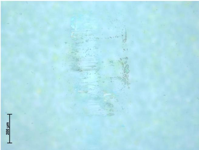
Fig. 9: Cracks for PEDOT samples tested for 2000 Cycles at a temperature of 23°C, a humidity of 30%, and a bending frequency of 60 cycles/min
