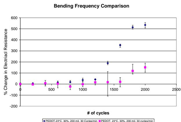
Fig.4: Effect of Bending Frequency on the percent change in electrical resistance of PEDOT, the experiments were conducted at a temperature of 23°C, a humidity of 30%, a bending diameter of 200 mil.
