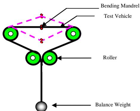
Fig. 2: Schematic of the fatigue tester
