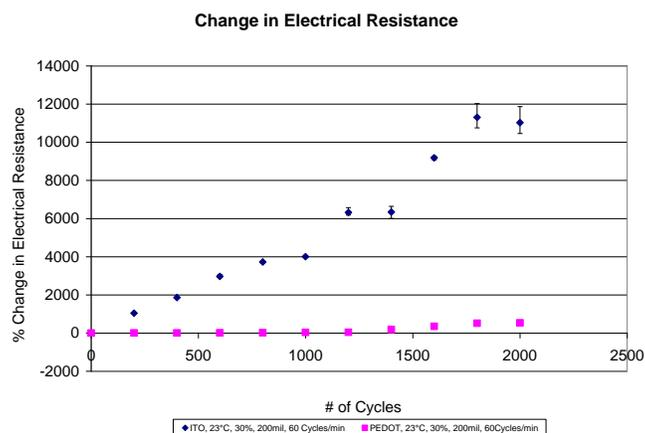
Fig. 3: Effect of material (PEDOT and ITO) on the percent change in electrical resistance, the experiments were conducted at a temperature of 23°C, a relative humidity of 30%, and a bending diameter of 200 mil, and a bending frequency of 60 cycles/minute
