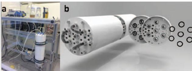
Fig. 3. Continuous formulation platform (a), the mixing mechanism (b).
