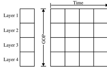
Figure 2. Encoding Group of Pictures on Layers.
