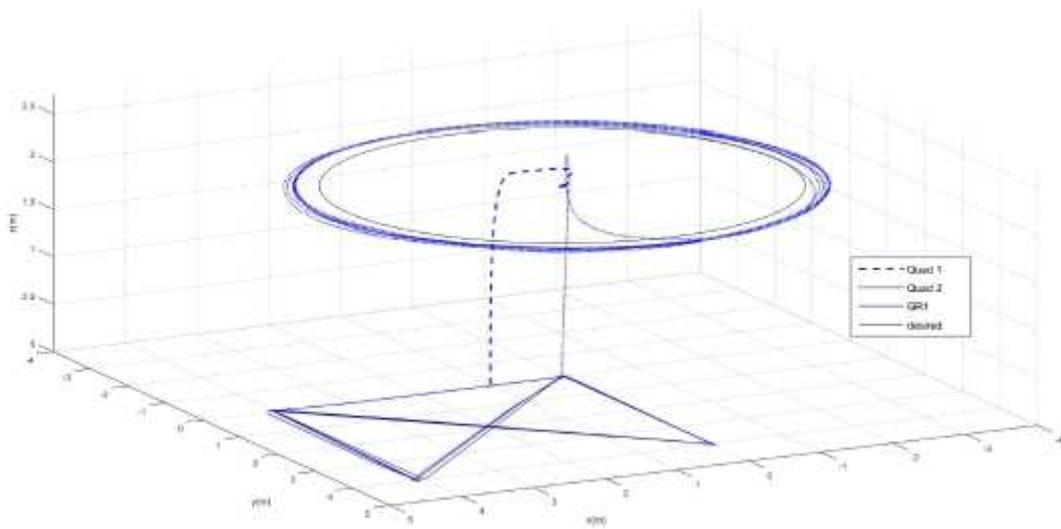
To ensure the validity of the used PID controllers in the proposed robots, external disturbances as a random form signals were carried out on each robot. These signals are applied on all axes in body frame of each robot with a value range of  $(-0.4 \text{ _ } 0.4) \text{ N}$ .
