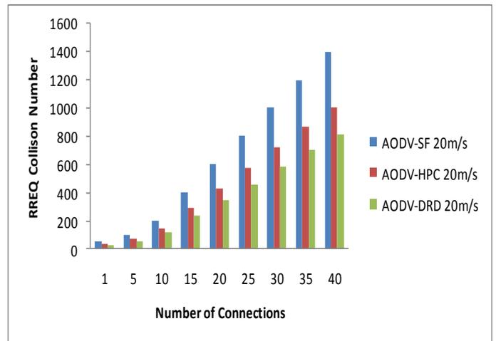
Figure 7: RREQ collision No vs. No of connections.
