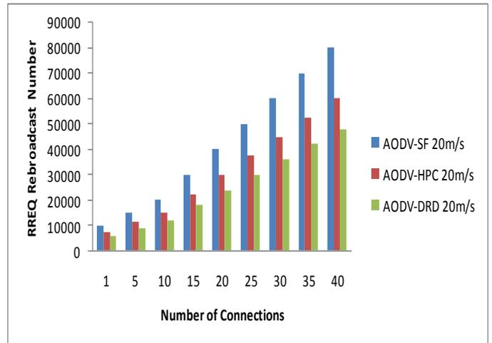
Figure6: RREQ Rebroadcast No vs. No of nodes.
