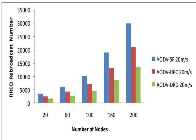
Figure 5: RREQ Rebroadcast No vs. No of connections.
