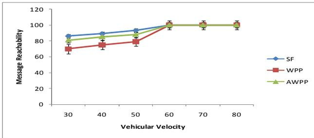
Figure 6: The R of three broadcast protocols vs vehicular velocity.
