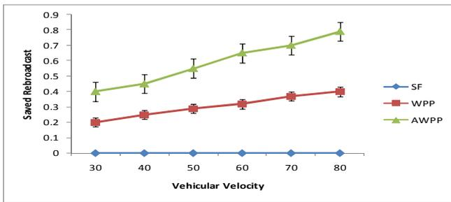
Figure 5: The SR of three broadcast protocols vs vehicular velocity.
