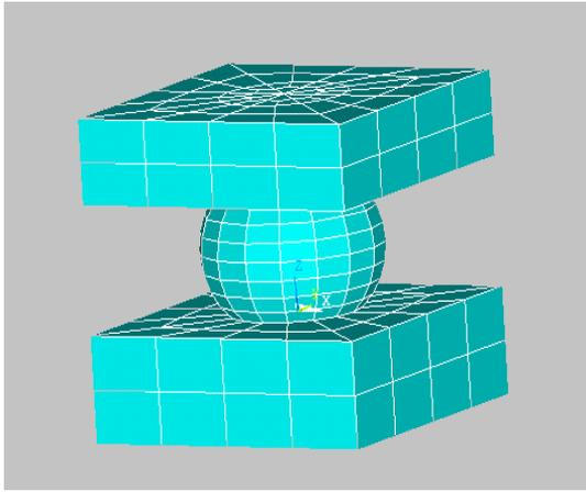
Figure 2. Typical solder joint unit.
