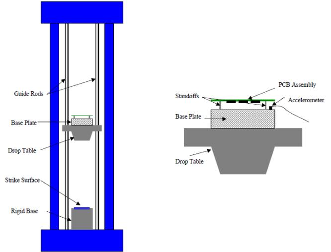
Figure 4. Schematic of JEDEC Drop Test [1].
