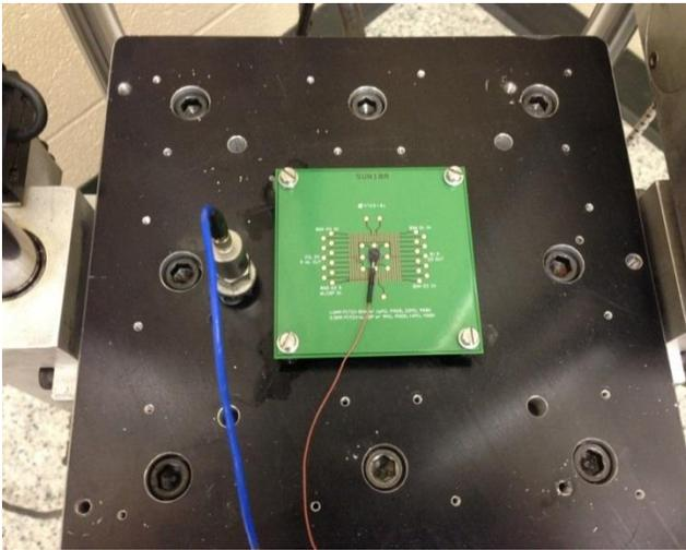
**Figure 1. Experimental setup of assembly (face down) mounted to the drop table. Two reference accelerometers are shown.**
