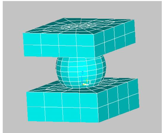
**Figure 2. Typical solder joint unit.**
