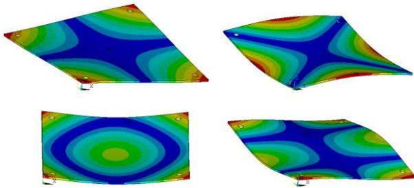
Figure 4. Unpopulated PCB Free Boundary conditions mode shapes (1<sup>st</sup>: top left, 2<sup>nd</sup>: top right, 3<sup>rd</sup>: bottom left, 4<sup>th</sup>: bottom right).
