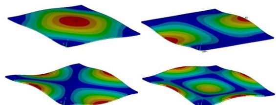
Figure 5. Unpopulated PCB Fixed Boundary conditions mode shapes (1<sup>st</sup>: top left, 2<sup>nd</sup>: top right, 3<sup>rd</sup>: bottom left, 4<sup>th</sup>: bottom right).
