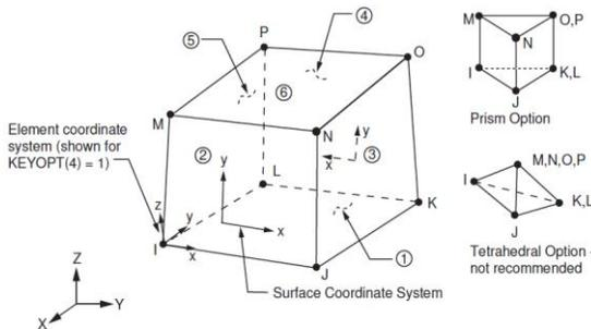
**Figure 1. ANSYS Solid45 3D element [10].**
