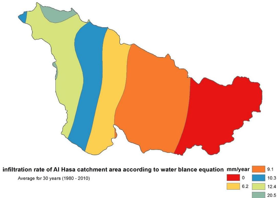
Fig. 5: The groundwater recharge zones that were estimated according to water balance equation and by overlaying method in GIS.
