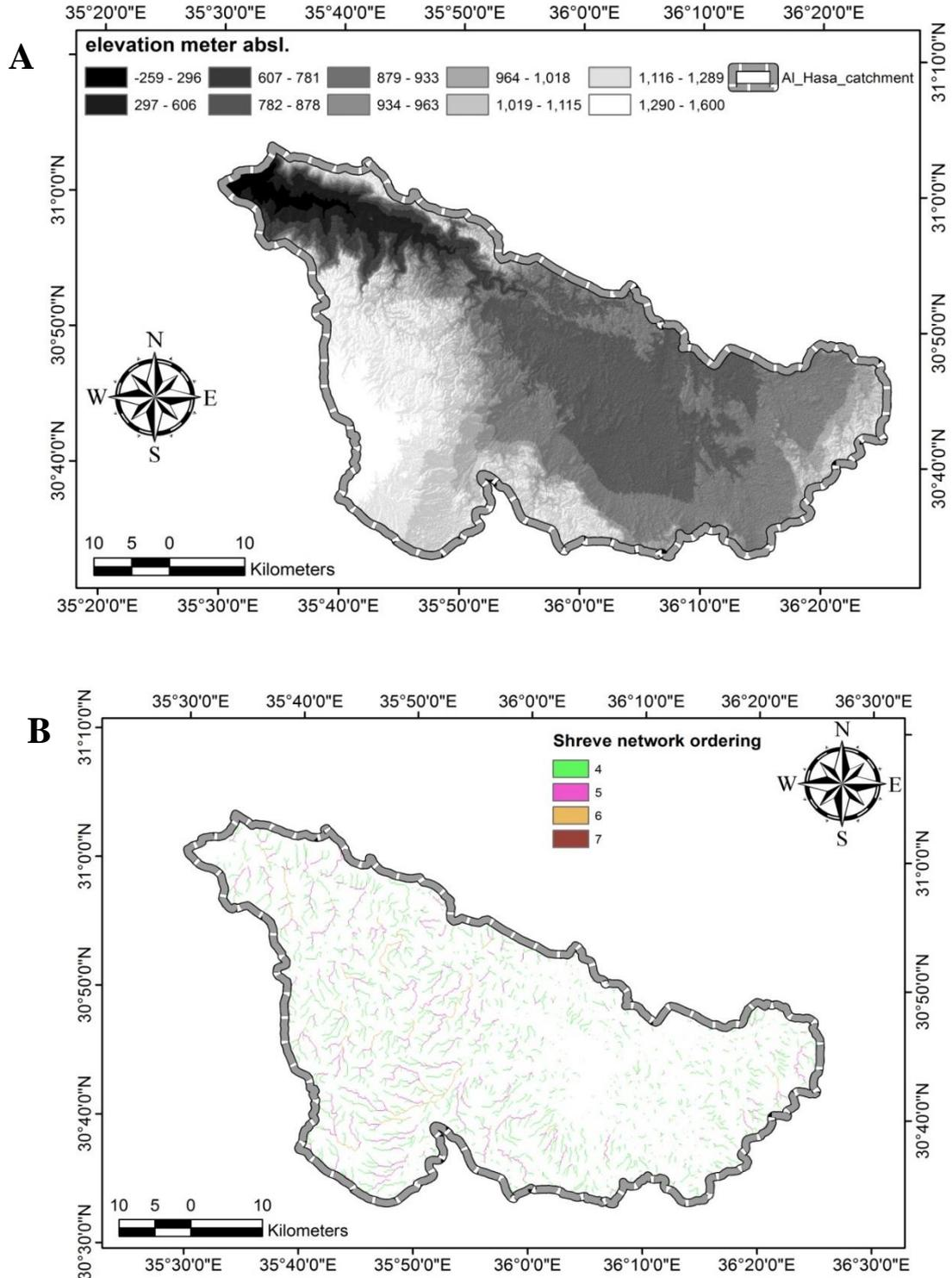
Fig. 3: The DEM of the study area (A) and the extracted drainage network (B).
