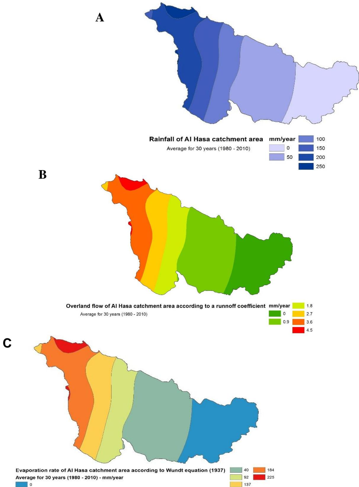
Fig. 2: The layers that we used to generate our analytical model. A) is the rainfall pattern that generated by interpolate the rainfall values by ArcGIS 10.3. B) is the overland follow for each rainfall pattern according to the runoff coefficient. C) is evaporation that were estimated according to wundt equation.
