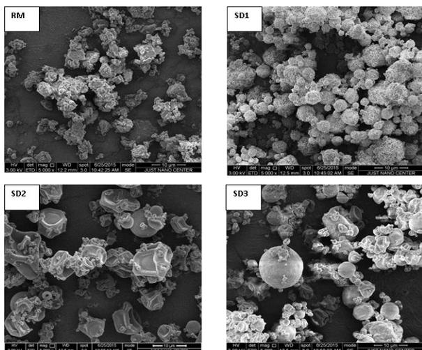
**Figure 1: SEM images of spironolactone raw material (RM) and spray dried batches SD1–SD3 (Table 1)**
