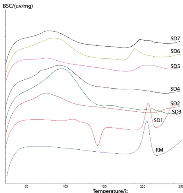
**Figure 3: DSC thermograms for co-spray dried products**
