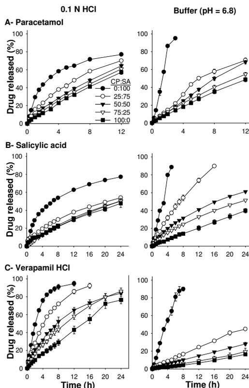
**Fig. 1.** Release profiles of paracetamol (A), salicylic acid (B) and verapamil HCl (C) from matrices containing Carbopol® 971P, CP, and sodium alginate, SA, at different ratios in 0.1 N HCl (left) and phosphate buffer, pH = 6.8 (right). Symbols are according to paracetamol profiles in 0.1 N HCl.
