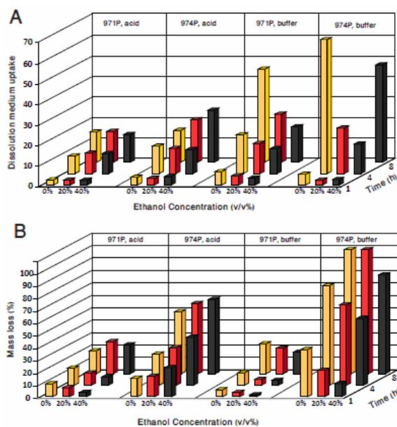
**Fig. 2.** Dissolution medium uptake (A) and mass loss (B) for CP 971P and 974P compacts in hydro-ethanolic acidic and buffered media.
