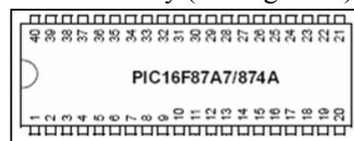
Fig.4 Microchip PIC 16F877 Microcontroller [6].
