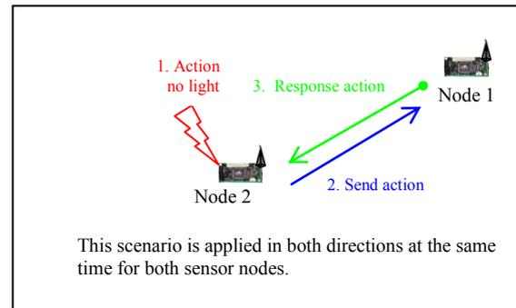
Fig. 7 Light Monitoring Application Communication Scenario
