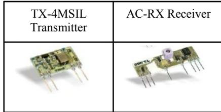
Fig. 5 AM Aural Transceiver Module [7].
