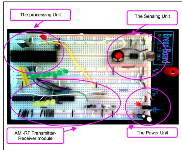
Fig. 6.b Implemented Sensor Node
