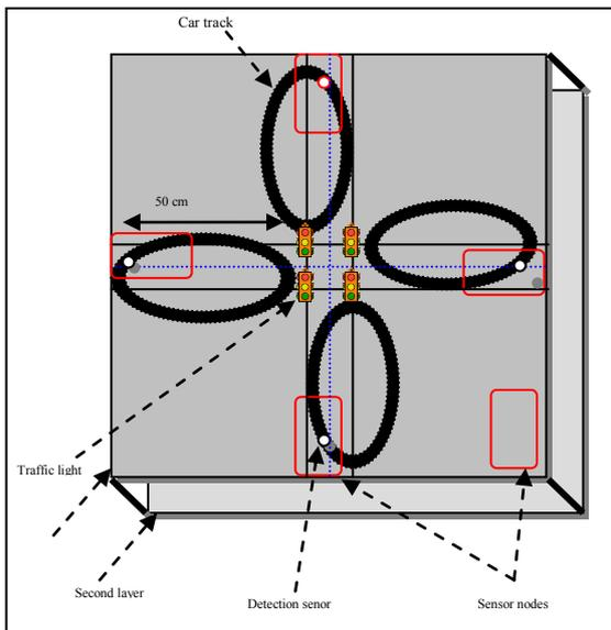
Fig.12 Traffic Light Control Architecture
