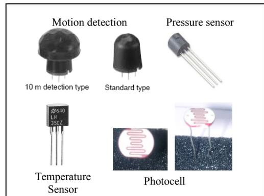
Fig.3 On Board Sensors
