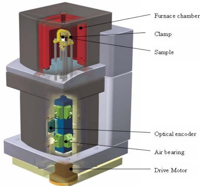
Figure 1. Schematic of TA instruments model Q800 DMA [14]
