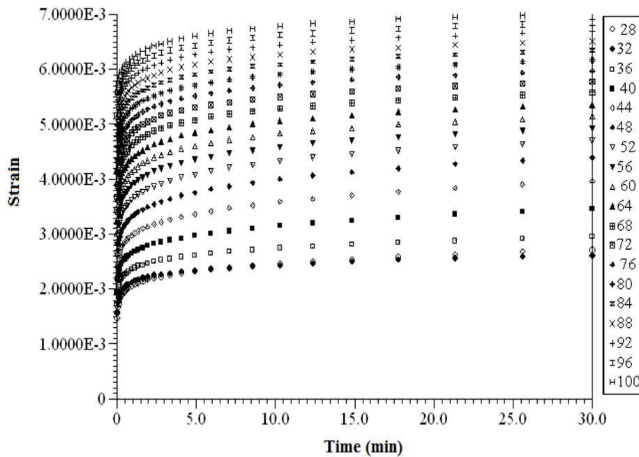
Figure 18. Typical DMA plot of creep-strain for pure nylon 6,6 over 30 min at various temperatures ( $^{\circ}\text{C}$ )
