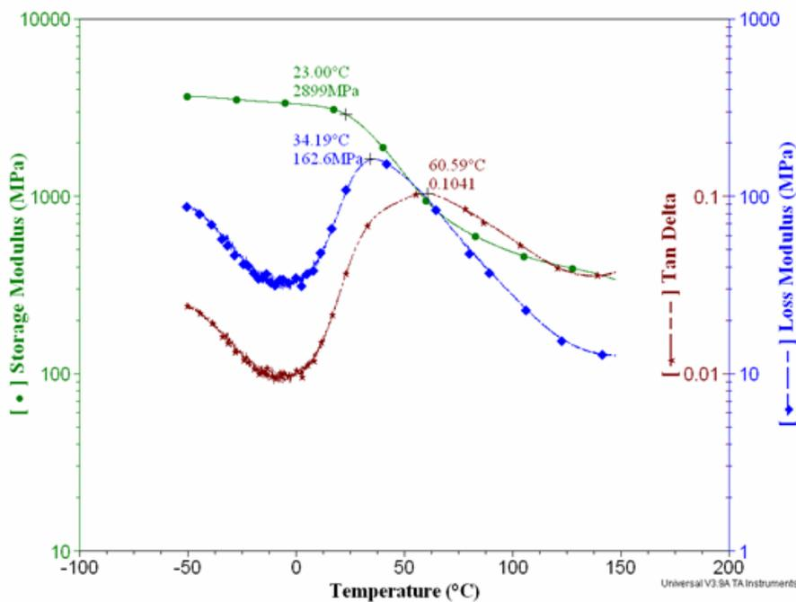
Figure 3. Dynamic modulus and damping for pure nylon 6,6
