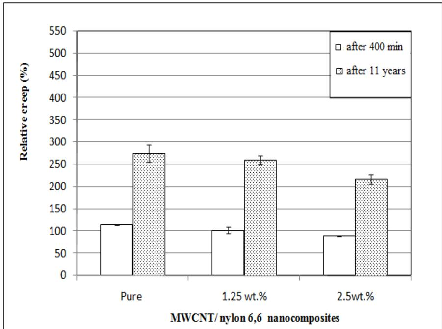
Figure 24. Relative creep for MWCNT /nylon6,6 nanocomposites generated from shifting of creep data at different temperatures to reference temperature (~ 28 to 30 °C )
