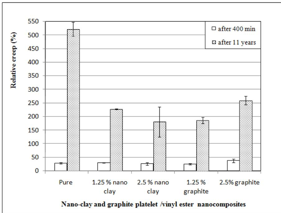
Figure 25. Relative creep for vinyl ester nano clay and graphite nanocomposites generated from shifting of creep data at different temperatures to reference temperature (~ 28 to 30 °C )
