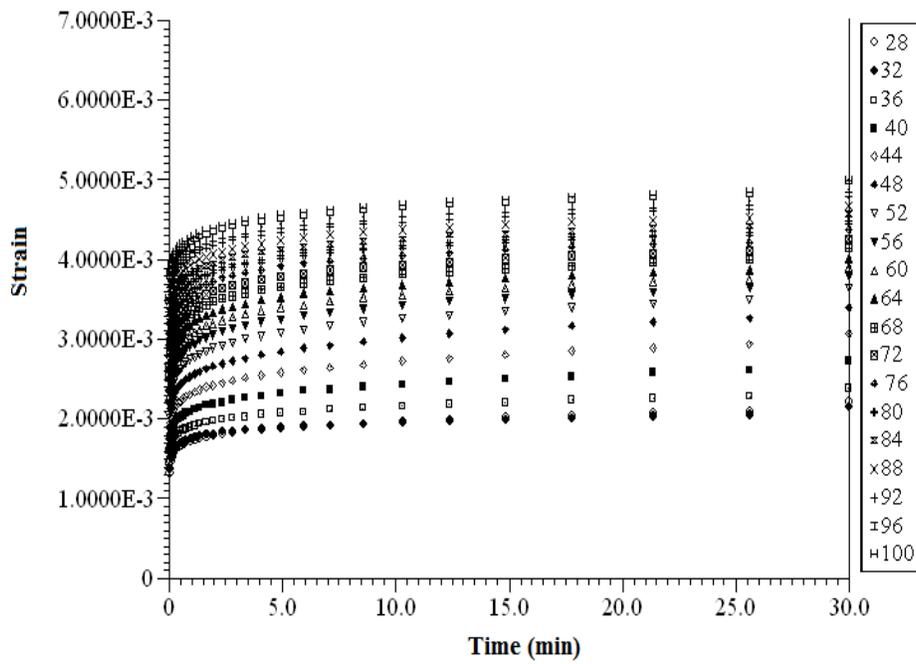
Figure 19. Typical DMA plot of creep-strain for 2.5 wt. percent MWCNT /nylon 6,6 over 30 min at various temperatures (°C)
