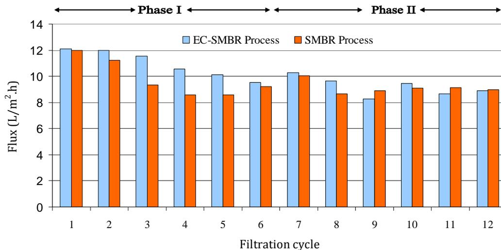
**Figure 4. Average permeate fluxes from EC-SMBR and SMBR processes during the two experimental phases**
