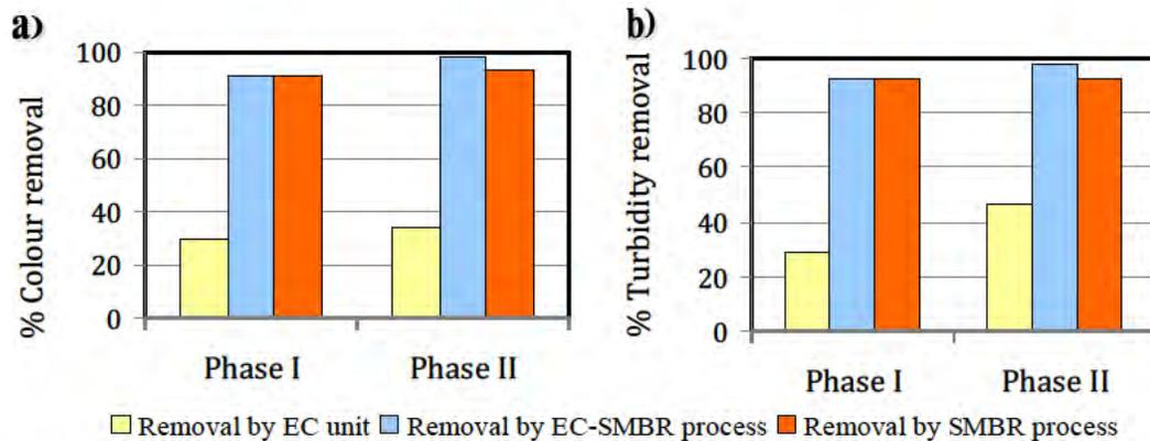
**Figure 2. Average percentage removal efficiencies of the EC unit, EC-SMBR process and SMBR alone during the two experimental phases: a) % Colour removal and b) % Turbidity removal**
