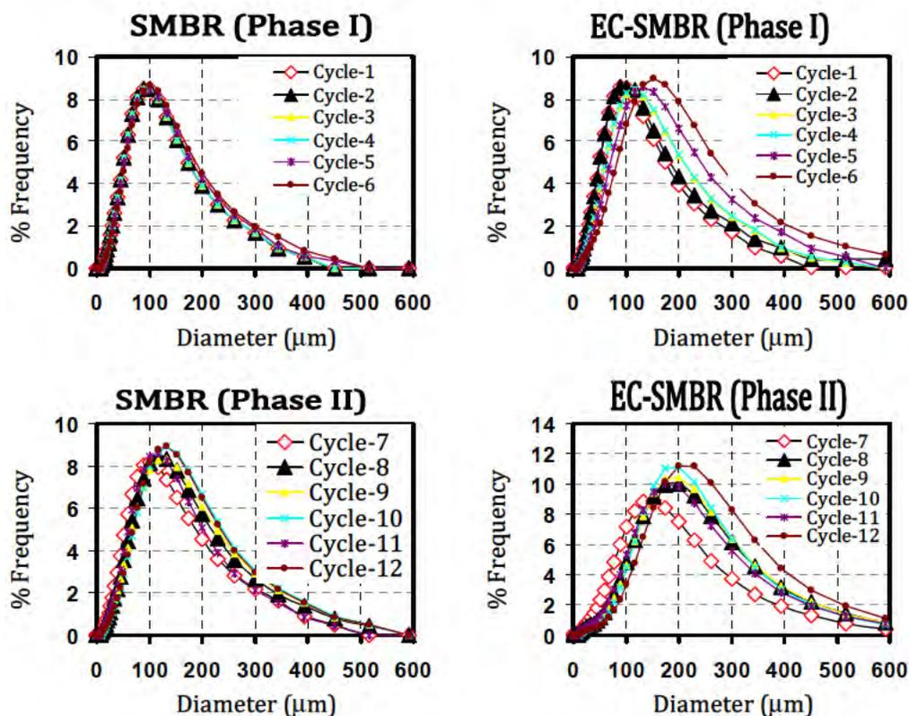
**Figure 5. Variations of the particles size distribution of sludge suspensions in SMBR and EC-SMBR processes during twelve cycles of the two experimental phases**
