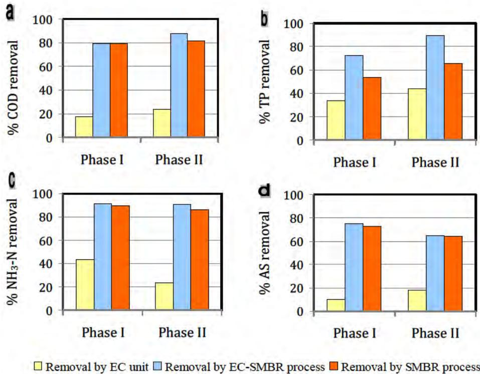
**Figure 3. Average percentage removal efficiencies of the EC unit, EC-SMBR process and SMBR alone during the two experimental phases: a) % COD removal, b) % Po<sub>4</sub><sup>3-</sup> removal, c) % NH<sub>3</sub>-N removal and d) Anionic surfactants (AS) removal**
