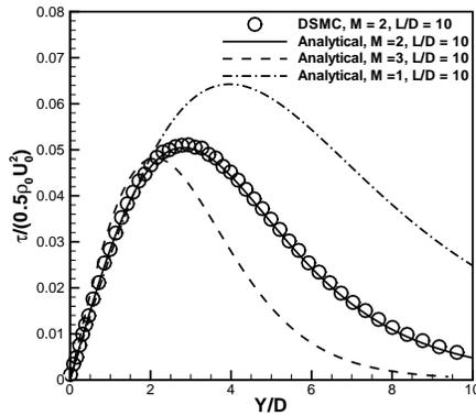
**FIGURE 3.** Profiles of normalized shear stress on the plate surface,  $\tau_{xy}/(\rho_0 U_0^2/2)$ , collisionless,  $L/D = 10$ .
