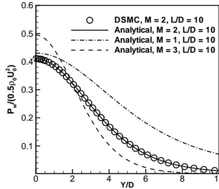
**FIGURE 2.** Profiles of normalized pressure on the plate surface,  $P(L-, y)/(\rho_0 U_0^2/2)$ , collisionless,  $L/D = 10$ .
