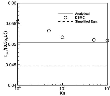
**FIGURE 5.** Normalized maximum shear stress on the plate surface for different Kn number,  $M_0 = 2$ ,  $L/D = 10$ .
