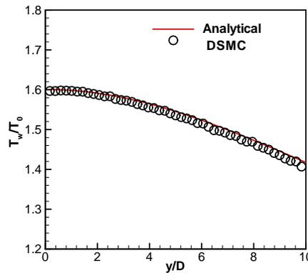
**FIGURE 4.** Profiles of normalized near-plate temperature,  $T_w/T_0$ , collisionless,  $M_0 = 2, L/D = 10$ .
