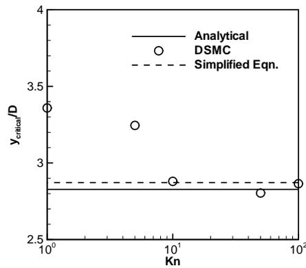
**FIGURE 6.** Normalized critical plate locations with the maximum shear stress for different Kn number,  $M_0 = 2$ .
