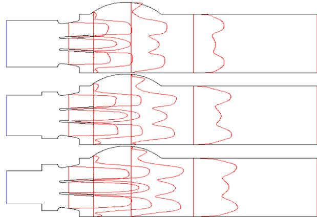
Figure 5: The velocity profiles at 1D, 2D, 3D and leaflets edges downstream of normal BMHV with different cases of SAS severity.
