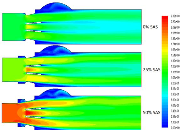
Figure 3: Contours of velocity magnitude (m/s) for normal BMHV with different cases of SAS severity at normal flowrate ( $Q=5.723 \times 10^{-4}$  (m<sup>3</sup>/s).
