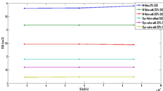
Figure 8: The relationship between EOA and flowrate for normal and dysfunction BMHV with different cases of SAS severity.
