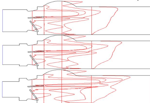
Figure 6: The velocity profiles at 1D, 2D, 3D and leaflets edges downstream of dysfunctional BMHV with different cases of SAS severity.
