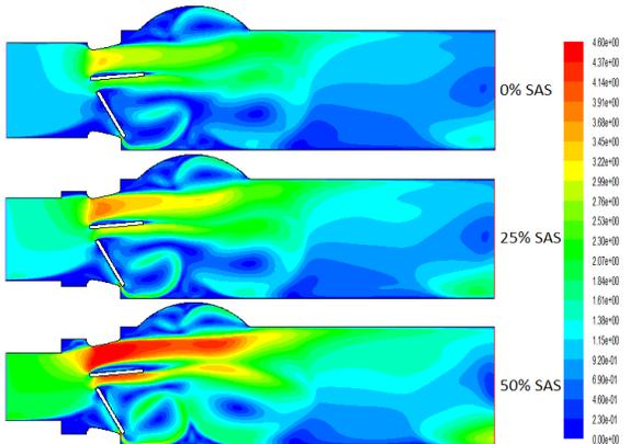
Figure 4: Contours of velocity magnitude (m/s) for Dysfunctional BMHV with different cases of SAS severity at normal flowrate ( $Q=5.723 \times 10^{-4}$  (m<sup>3</sup>/s).
