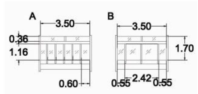
Figure 2: A) Vertical shading elements placed at 60 cm apart, B) A shading element added at the center between two existing shading elements.
