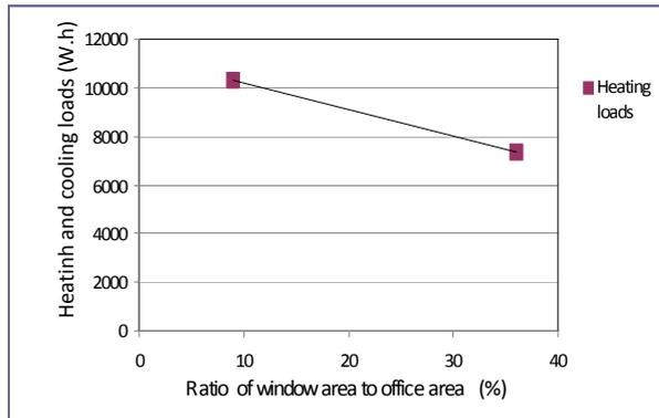
Figure 3: Heating loads for offices and the ratio of window area to office area (Note: all offices oriented south).
