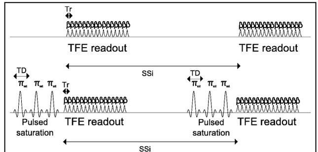
Fig. 1: The MT-RAGE sequence with MT<sub>on</sub> (top) and MT<sub>off</sub> (bottom) versions. The Shot-to-shot interval was kept at 10seconds to allow the longitudinal magnetization to fully recover before the next pulse train.
