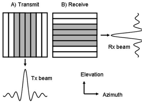
Fig. 1. 3-D scanning process of the dual-layer transducer
