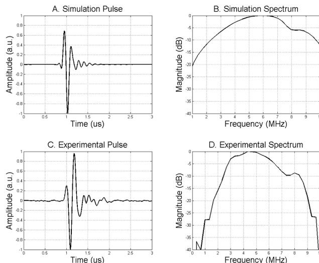
Figure 5. Simulated and experimental pulse and spectra of the dual-layer transducer.
