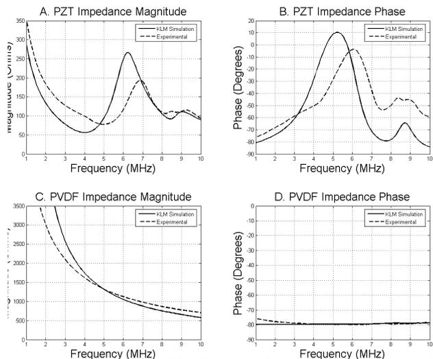
Figure 4. Simulated (solid lines) and experimental (dashed lines) impedance measurements of PZT and PVDF layers.
