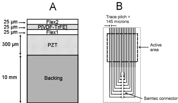
Fig. 2 Acoustic stack of the dual-layer transducer and schematic of the flexible circuits.
