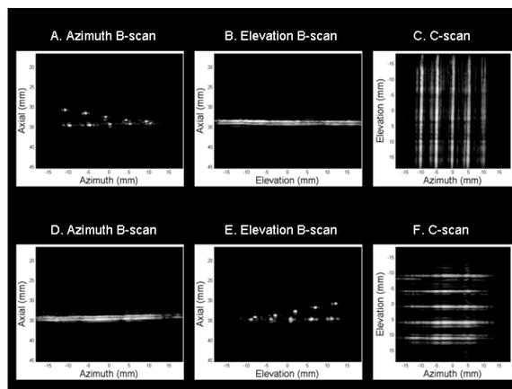
Figure 6. Experimental axial wire target images with short axis in azimuth (A-C) and short axis in elevation (D-F). All
