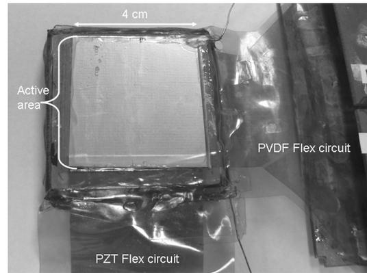
Figure 3. Photo of the prototype dual-layer transducer
