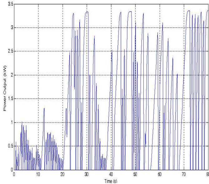
**Figure 5: FC output versus time for LP FC model on daytime drive cycle**
