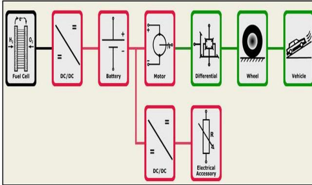
**Figure 3: PSAT component configuration for series fuel cell hybrid rickshaw**
