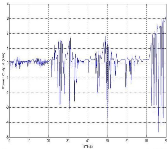
**Figure 6: Battery output versus time for LP FC model on daytime drive cycle**
