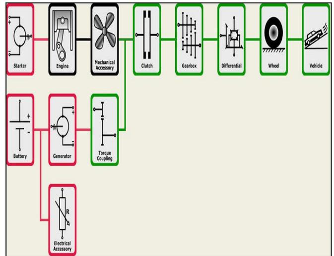
Figure 2: PSAT component configuration for conventional rickshaw
