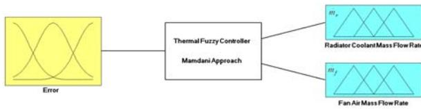
Figure 3. Input/outputs of fuzzy logic control
