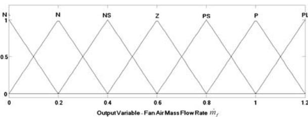
Figure 6. Fan air mass flow rate membership functions
