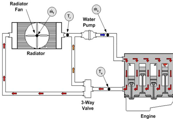
Figure 1. Advanced cooling system with electrical-actuated components.
