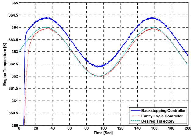
Figure 7: Simulated engine temperature response (Case I)
