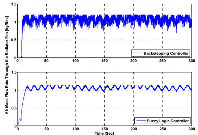
Figure 12: Simulated air mass flow rate through the radiator fan (Case II)
