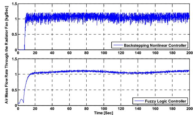
Figure 9: Simulated air mass flow rate through the radiator fan (Case I)
