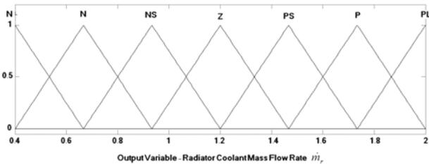
Figure 5. Radiator coolant mass flow rate membership functions
