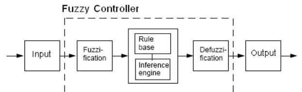
Figure 2. Structure of fuzzy logic control
