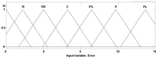
Figure 4. Engine temperature tracking error membership functions
