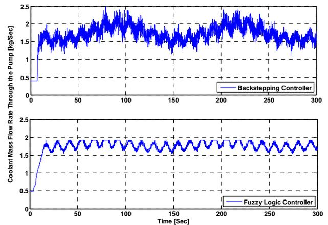
Figure 11: Simulated coolant mass flow rate through the pump (Case II)
