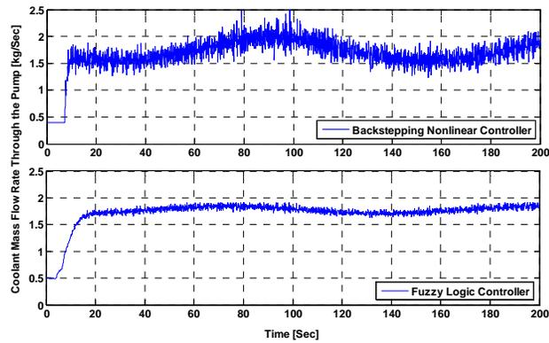
Figure 8: Simulated coolant mass flow rate through the pump (Case I)
