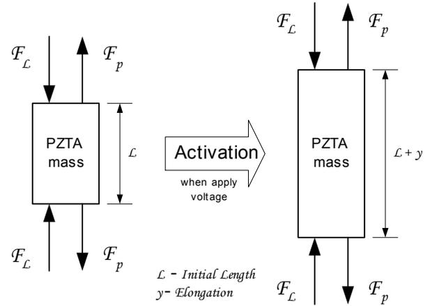
**Figure 1:** PZTA elongation induced by applied voltage
