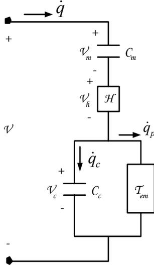
**Figure 2:** PZTA equivalent circuit model
