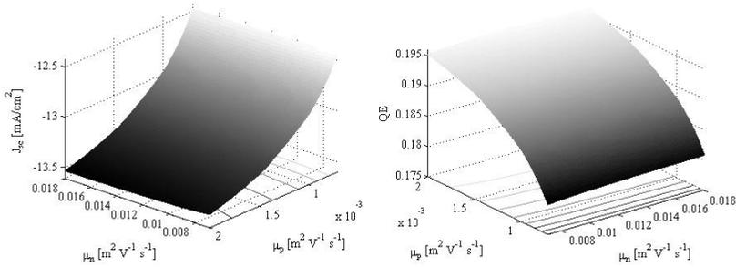
Figure 5: Comparison between the effects of electron and hole mobilities on short circuit current and quantum efficiency.
