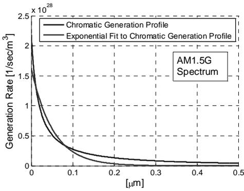
Figure 1: Chromatic generation profiles and its exponential fitting over position.
