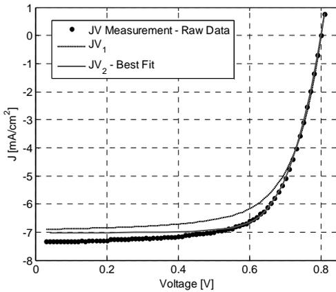
Figure 2: Comparison between an a-Si test cell and the model. Results, under STCs.
