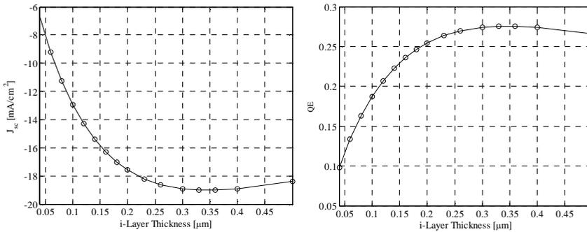
Figure 6: Effect of i-layer thickness on QE, under zero external bias conditions.
