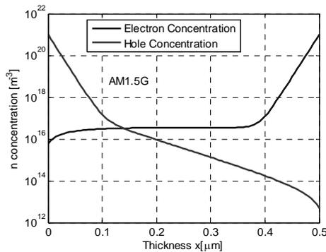
Figure 3: Free carrier distribution on a p-i-n junction, with a non-uniform excitation through the p layer, under no external bias.
