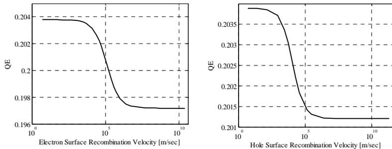
Figure 4: Comparison between the effects of surface recombination velocities of electron and holes on the quantum efficiency.
