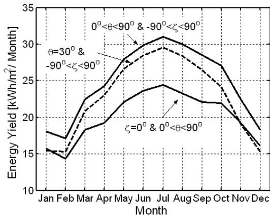
**Fig. 10. Comparison of the energy yield of the two-axis (variable  $\theta$  and  $\zeta$ ) and the one-axis (fixing  $\zeta$  or  $\theta$ ) tracking of PV systems. The tracking about azimuth or the inclination shows comparable results to each other in the winter months.**
