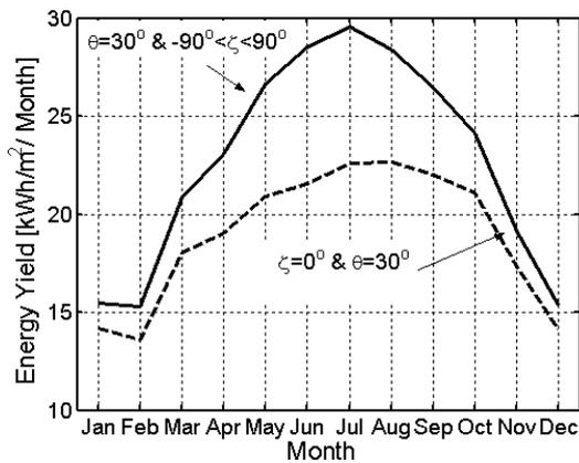
Fig. 7. Energy yield of fixed (fixing both  $\zeta$  and  $\theta$ ) and one-axis (fixing  $\theta$  and varying  $\zeta$ ) of PV systems for each month. The maximum energy yield occurs in also July for both curves. The gain of such tracking over the fixed one is 20.12%.
