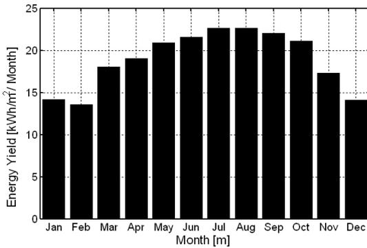
Fig. 3. Energy yield of the PV systems, the energy yield is  $227.1 \text{ kWh/m}^2/\text{year}$ .
