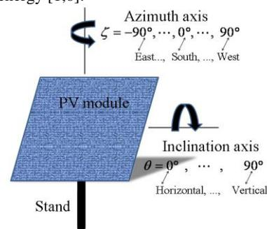
**Fig. 1. Two-axis tracking configuration where the PV module rotates about its axes (inclination and azimuth) by a controllable gear.**
