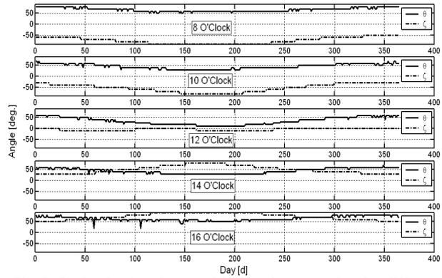
Fig. 8. Optimal azimuth  $\zeta$  and inclination  $\theta$  angles for different times in the day over all the year.
