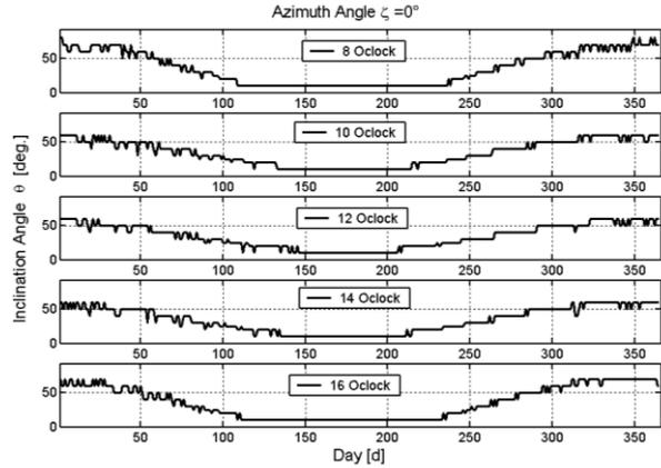
Fig. 4. Optimal inclination angles  $\theta$  for different times in the day over all the year while the azimuth angle is set to  $\zeta = 0^\circ$ .
