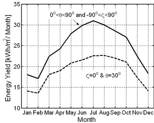
Fig. 9. Energy yield of fixed (fixing both  $\zeta$  and  $\theta$ ) and two-axis (varying both  $\theta$  and  $\zeta$ ) of PV systems for each month. The maximum energy yield occurs in also July for both lines. The gain of such tracking over the fixed one is 30.82%.
