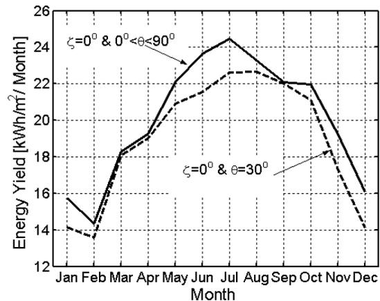
Fig. 5. Energy yield of fixed (fixing both  $\zeta$  and  $\theta$ ) and one-axis (fixing  $\zeta$  and varying  $\theta$ ) PV systems for each month. The maximum energy yield occurs in July for both lines. The gain of such tracking over the fixed one is  $5.87\%$ .
