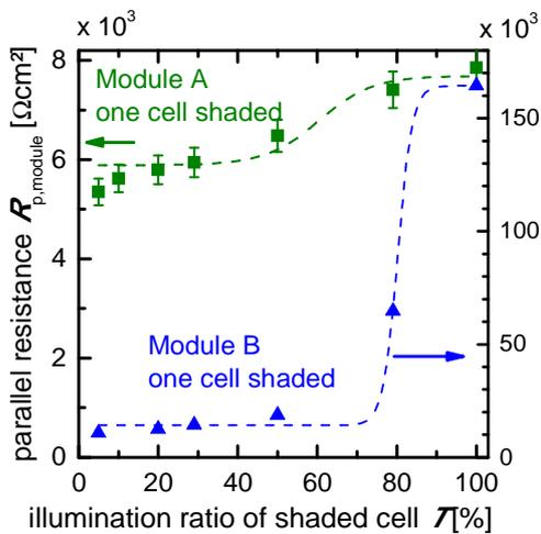
**Figure 4:** Measured  $R_{p,module}$  of two different types of commercially available mini-modules when different cells are shaded. The dashed lines are a guide to the eye and remind on the proposed model in section 2.3. Both examples do not show an increase of  $R_{p,module}$  at low  $T$  due to small  $\gamma$  at lower light intensities which is due to dominating shunts related to series interconnection of the solar cells.
