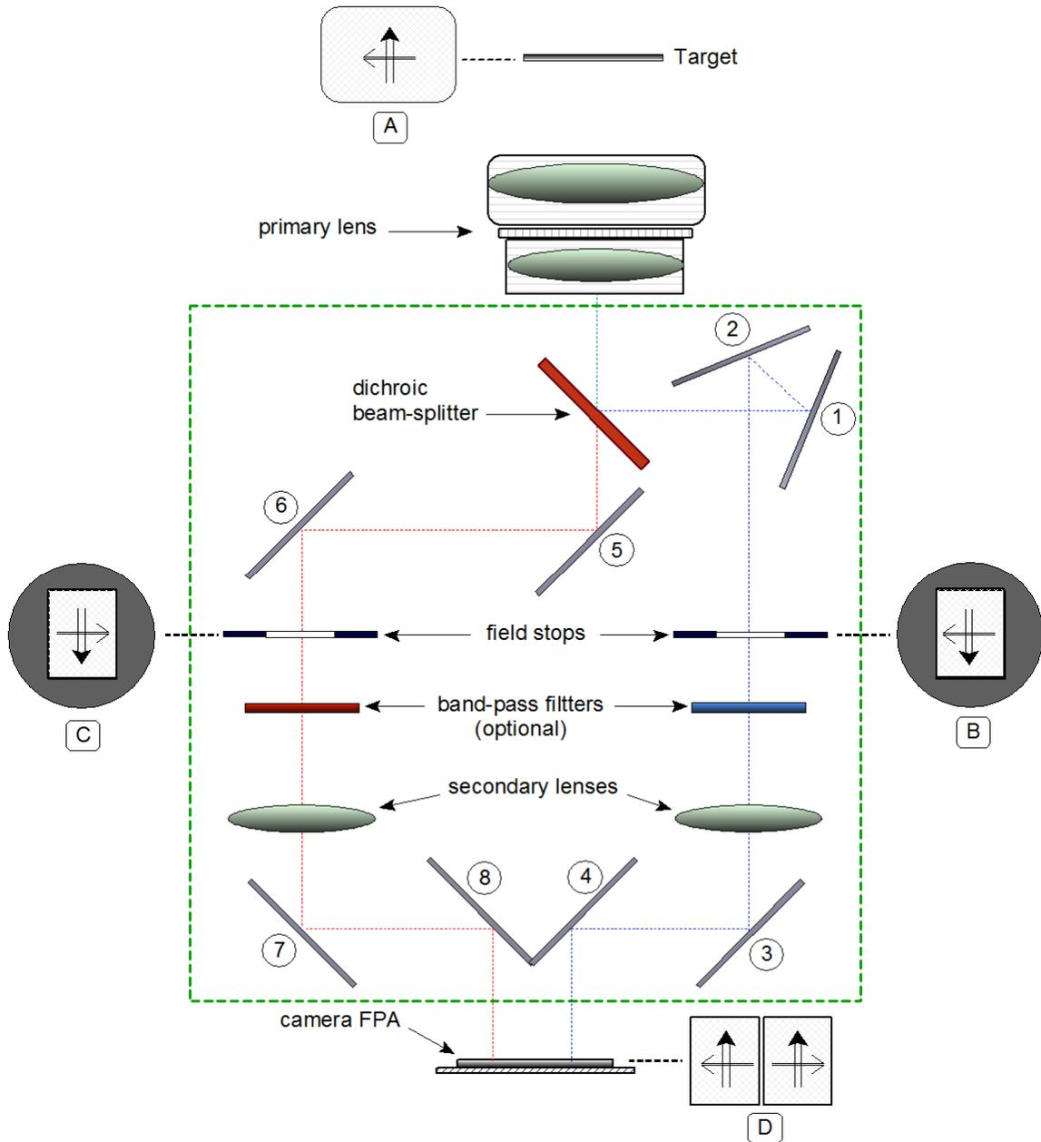
Fig. 3. The optical design of the new image splitter. (1 through 8: front surface reflection mirrors; A through D: illustrative rotated views of the target, RHS & LHS field stops at the intermediate real-image planes, and the real images projected on the FPA, respectively)
