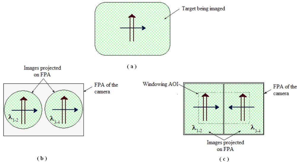
Fig. 2. Desired improvement to image-splitter; (a) The target that is being imaged, (b) The images projected on the camera FPA using the basic image splitter design, and (c) The images projected on the FPA of the camera using the new image splitter design.
