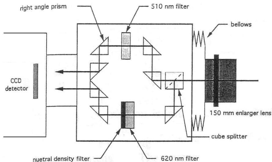
Fig. 1. Schematic of the optical image-splitter used for dual-wavelength imaging by Bizzak and Chyu [9].
