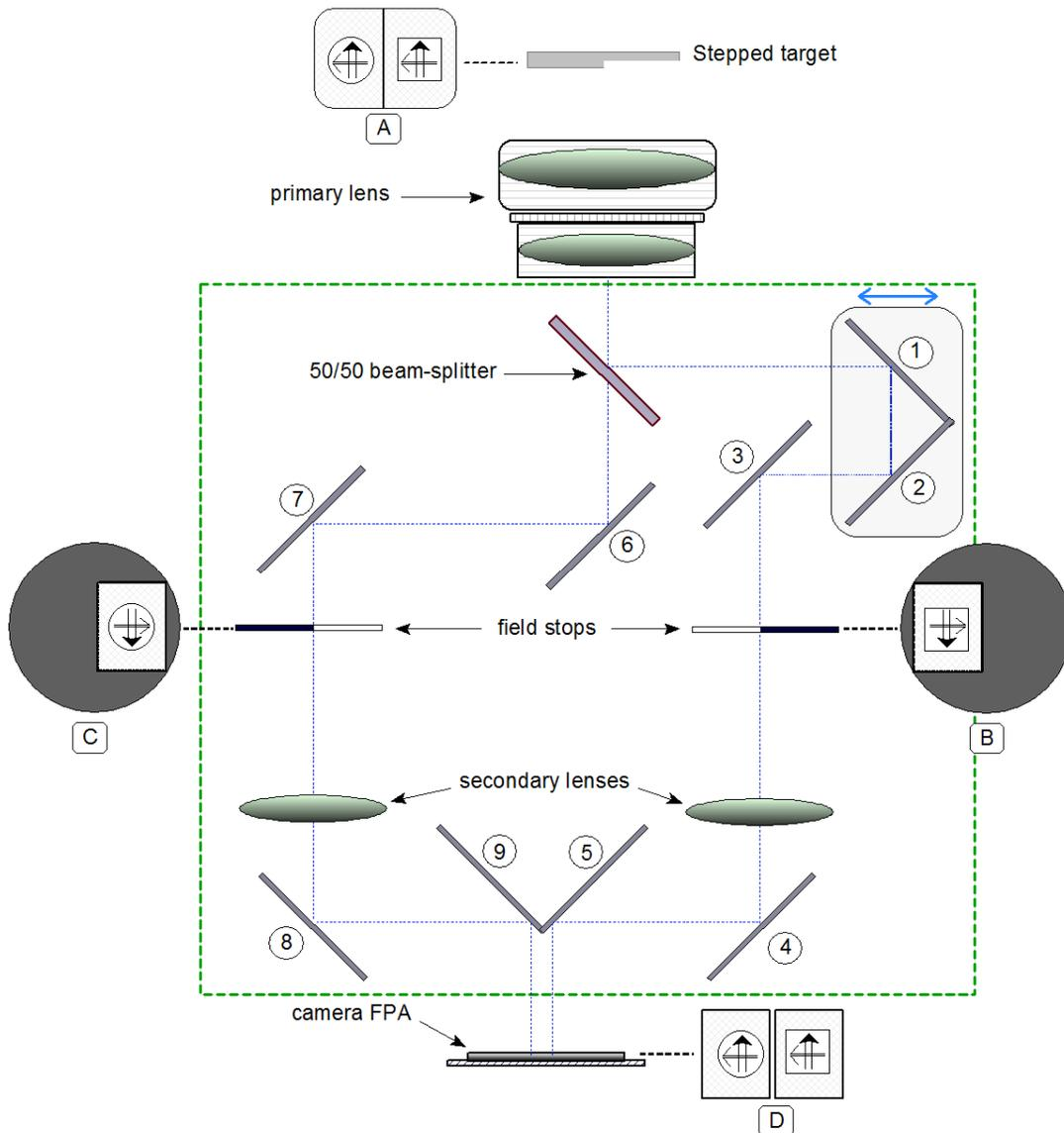
Fig. 4. The modified design for imaging stepped targets. (1 through 9: front surface reflection mirrors; A through D: illustrative rotated views of the target, RHS & LHS field stops at the intermediate real-image planes, and the real-images projected on the FPA, respectively)
