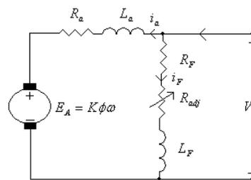
Fig. 1. Equivalent Circuit of DC Shunt Motor
