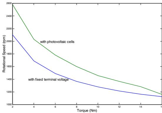
Fig. 14. Torque-speed characteristics of DC series motor with photovoltaic cells and fixed terminal voltage
