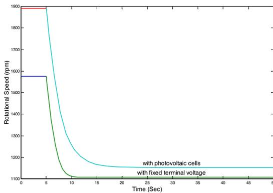
Fig. 7. Rotational speed of the DC series motor after a step increase in the load torque from 5Nm to 17Nm
