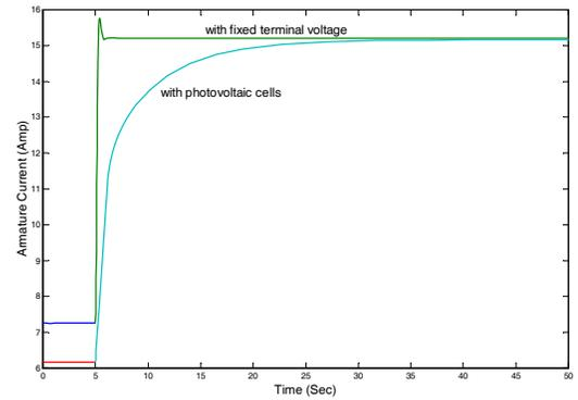
Fig. 4. Armature current of DC shunt motor after a step change on the load torque from 5Nm to 10.4Nm with a field resistance of  $100 \Omega$
