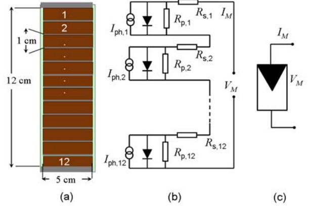
Fig. 1: Thin film amorphous silicon a-Si:H PV module consisting of 12 series-connected solar cells (a) and its equivalent circuit (b). For simplification, the symbol in (c) is used to represent the PV module. The effective area of the module is  $60 \text{ cm}^2$  where the area of each cell is  $5 \text{ cm}^2$ .
