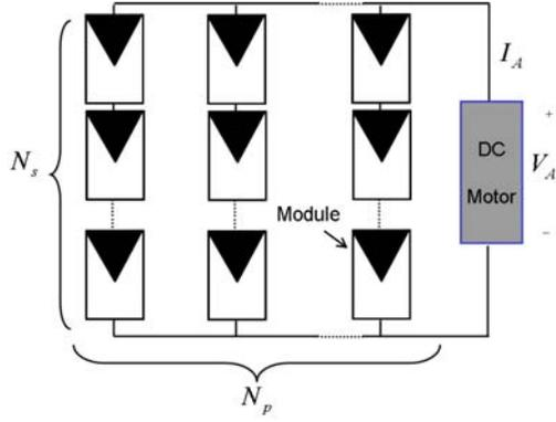
Fig. 2: A PV array consisting of  $N_s$  series- and  $N_p$  parallel-connected modules loaded by either dc motor shunt or series motor
