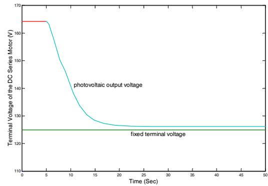
Fig. 8. Terminal voltage of the DC series motor (photovoltaic cells voltage) after a step increase in the load torque from 5Nm to 17Nm compared with the fixed voltage
