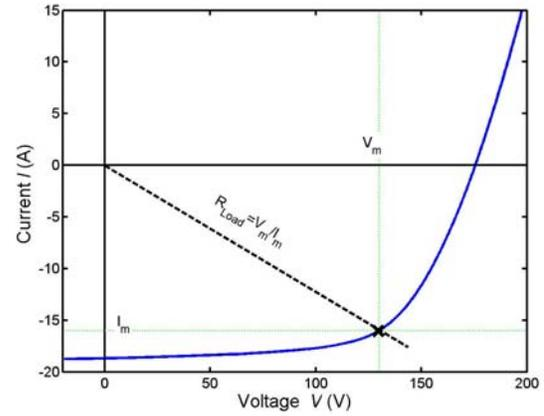
Fig. 3: Current/voltage characteristics of the designed PV array consisting of 19 series- and 252 parallel-connected modules.
