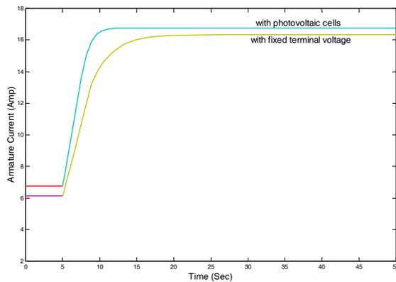
Fig. 6. Armature current of the DC series motor after a step increase in the load torque from 5Nm to 17Nm
