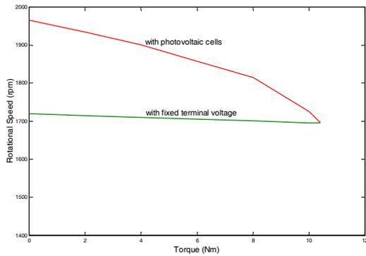
Fig. 13. Torque-speed characteristics of DC shunt motor with photovoltaic cells and fixed terminal voltage
