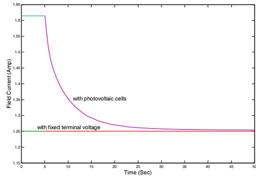
Fig. 3. Field current of DC shunt motor after a step change on the load torque from 5Nm to 10.4Nm with a field resistance of  $100 \Omega$
