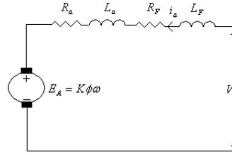
Fig. 2. Equivalent Circuit of DC Series Motor
