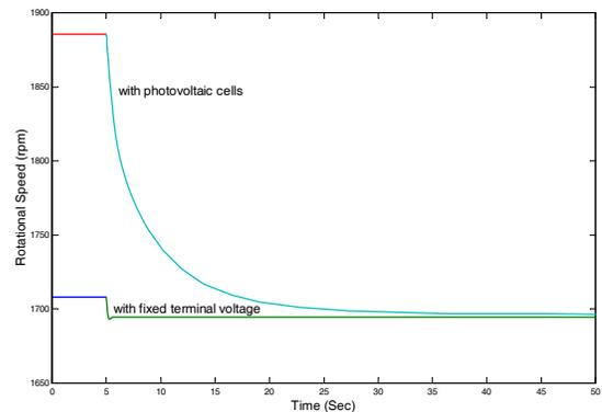
Fig. 5. Rotational speed of DC shunt motor after a step change on the load torque from 5Nm to 10.4Nm with a field resistance of  $100 \Omega$
