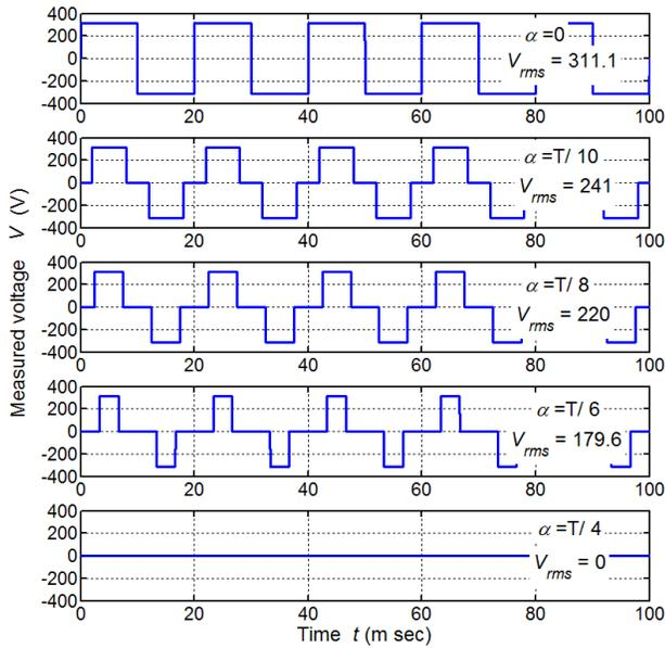
Figure 5: Measured voltage for different values of time delay  $\alpha$  and the resulting effective value  $V_{rms}$ .
