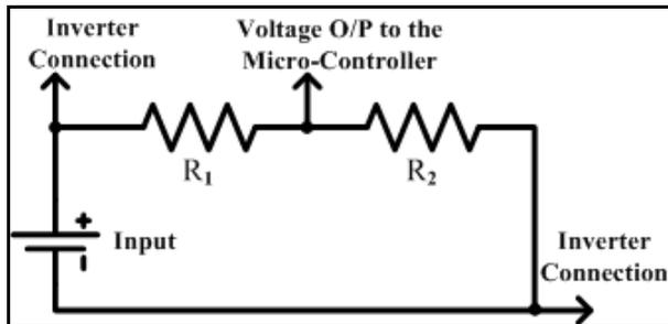
Figure 3: Voltage measuring circuit
