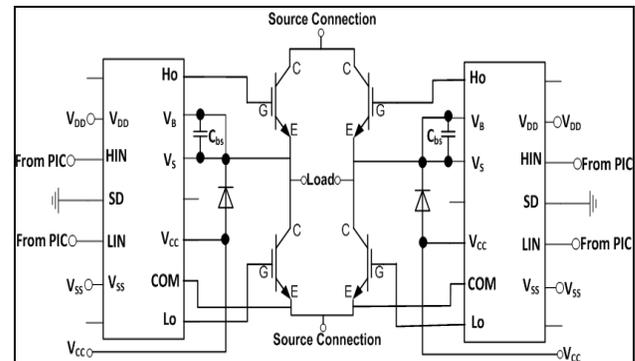
Figure 6: Gate Driver/Main Inverter Connection
