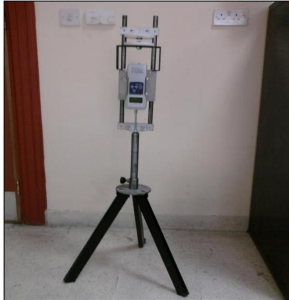
**Figure 1:** Custom-Designed Apparatus for Measuring Snap-Type Two-Handed Grip Strength
