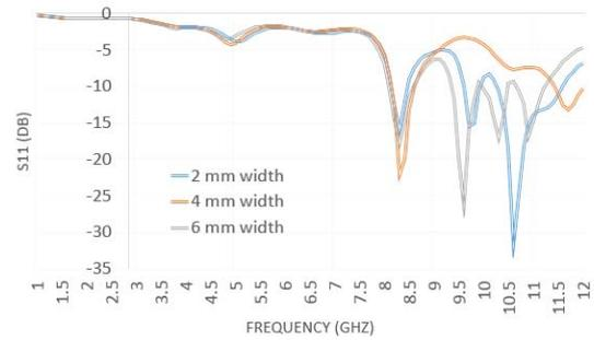
Fig. 3. Optimization of the slot width
