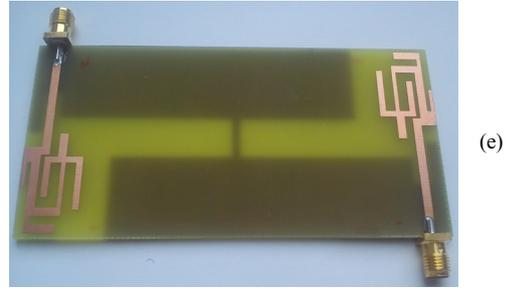
Fig. 1. Proposed MIMO antennas structure and dimensions (mm). (a) Front view (b) Details of single antenna element (c) Details of defected GND structure (d) Top view with the bottom layer showing through (e) Front view of fabricated antenna.
