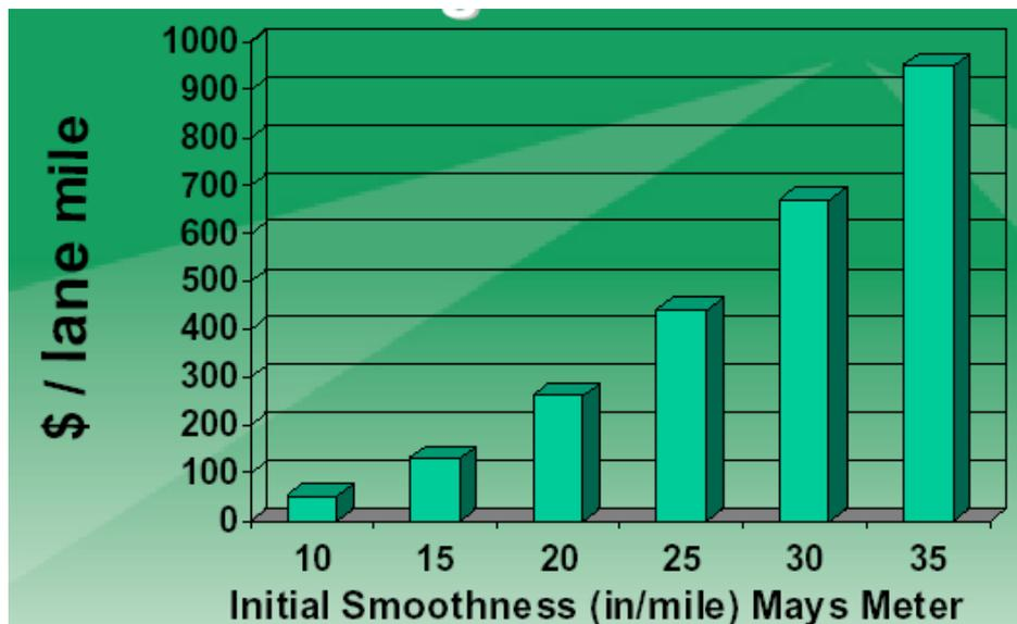
Figure 3: Effect of the initial pavement roughness on average annual maintenance cost (Janoff, 1990)
