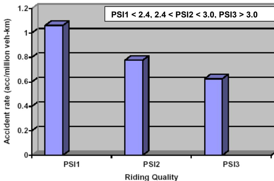
Figure 1: Effect of riding quality on vehicle accident rate (Bester, 2003)
