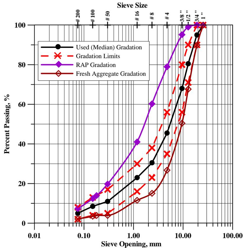
**Fig. 1. Ministry of Public Works & Housing specified gradation limits for heavy traffic loads wearing course, median gradation, RAP aggregate gradation, and added fresh aggregate gradation.**
