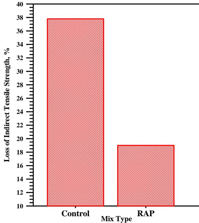
**Fig. 3. Loss of Indirect Tensile Strength (ITS) between mixture with fresh aggregates and asphalt, and mixture containing RAP.**
