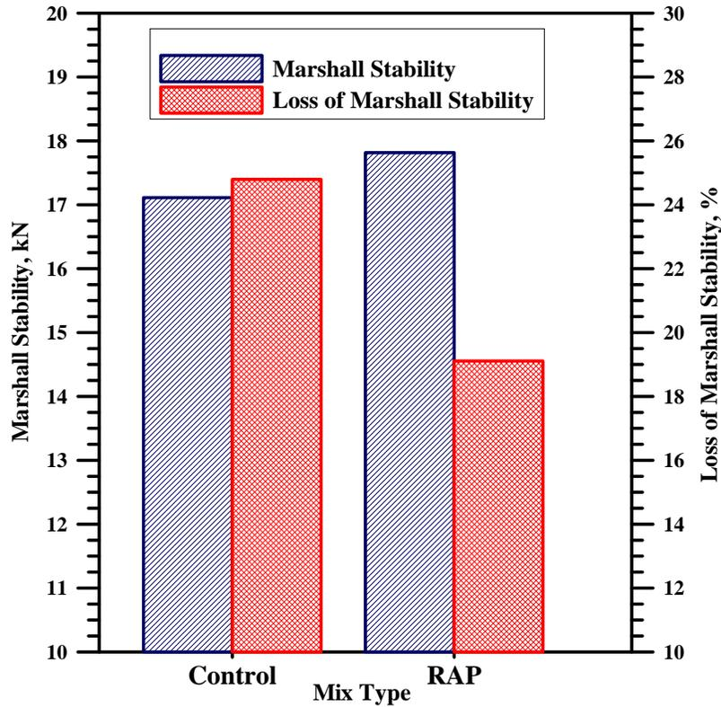
**Fig. 2. Marshall Stability and Loss of Marshall Stability between Control and Rap mixes.**
