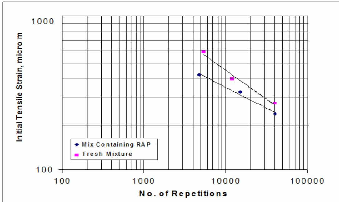
Fig. 5. Fatigue behavior for the two mixes @ 40°C
