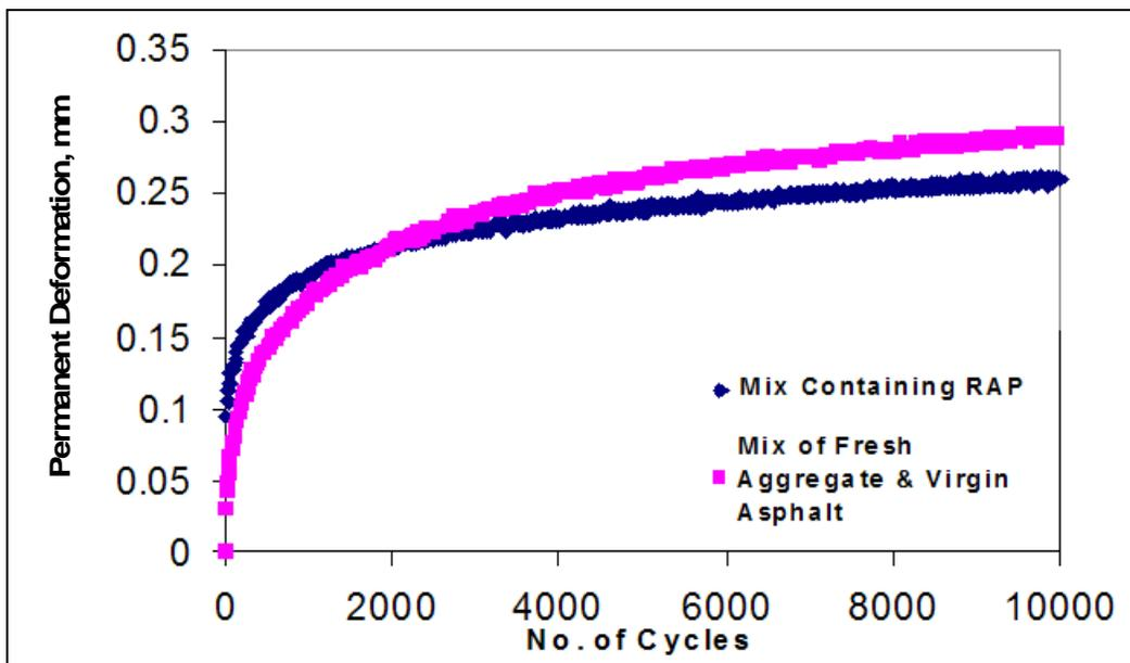
**Fig. 4 Average creep results of mixture with fresh aggregates and asphalt, and mixture containing RAP.**
