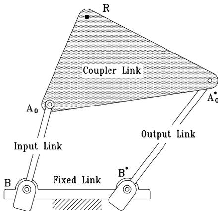
FIGURE 1. THE FOUR-BAR LINKAGE DESCRIPTION
