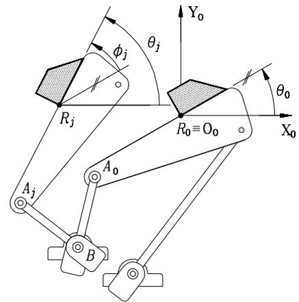
FIGURE 2. THE  $j$ th POSE OF A FOUR-BAR LINKAGE
