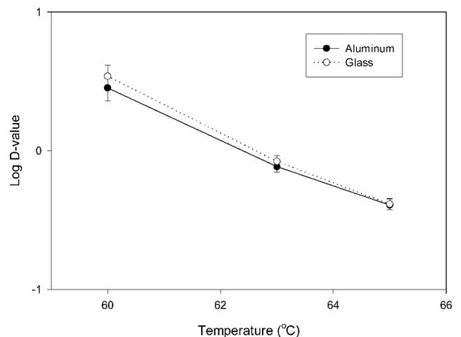
FIGURE 3. Thermal-death-time curves for *L. innocua* in salmon caviar heated in the glass and aluminum thermal-death-time tubes.
