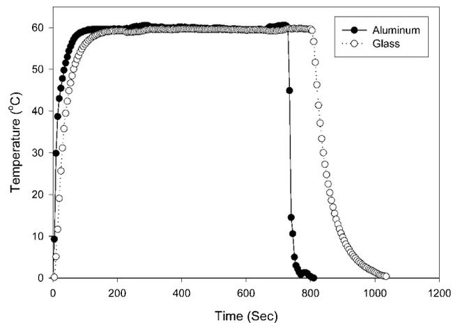
FIGURE 2. Effect of the glass and aluminum thermal-death-time tubes on heat penetration in salmon caviar at 60°C.
