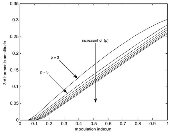
Fig.7 The third harmonic amplitudes for VPW,  $p=3, 5, \dots, 15$
