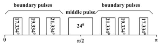
Fig.2 pulse widths for  $\delta = 140^\circ$  and  $p = 7$ .
