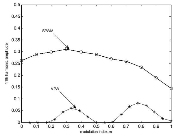
Fig.6 The 11<sup>th</sup> harmonic amplitude for VPW and SPWM techniques,  $p=5$
