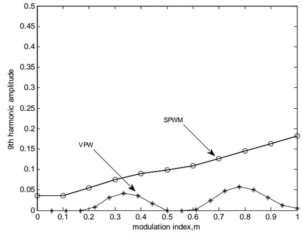
Fig.5 The 9<sup>th</sup> harmonic amplitude for VPW and SPWM techniques,  $p=5$
