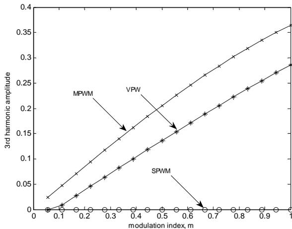
Fig.4 The 3<sup>rd</sup> harmonic amplitude for VPW technique and conventional techniques,  $p=5$
