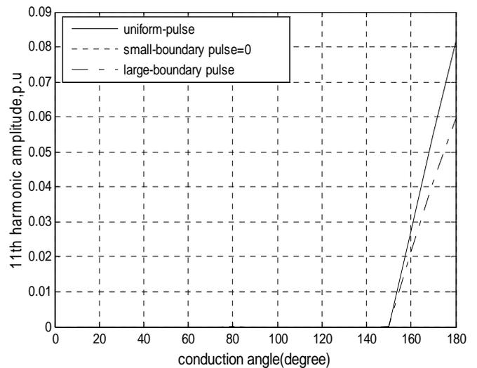
Figure.5 11th harmonic amplitude for different techniques
