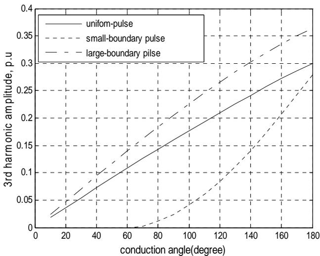
Figure.3 3rd harmonic amplitude for different techniques
