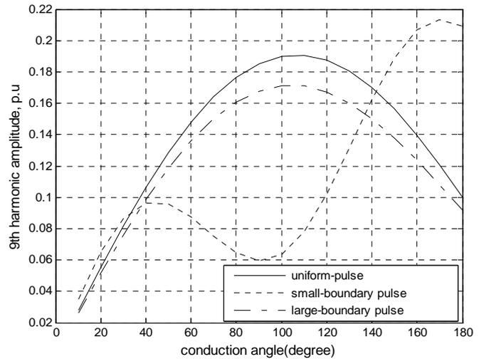
Figure.4 9th harmonic amplitude for different techniques
