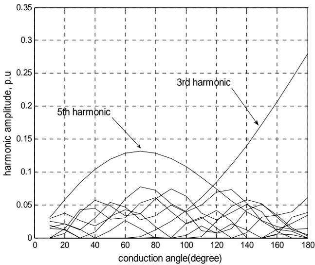
Figure.2 Harmonic profile for small-boundary pulse-width technique
