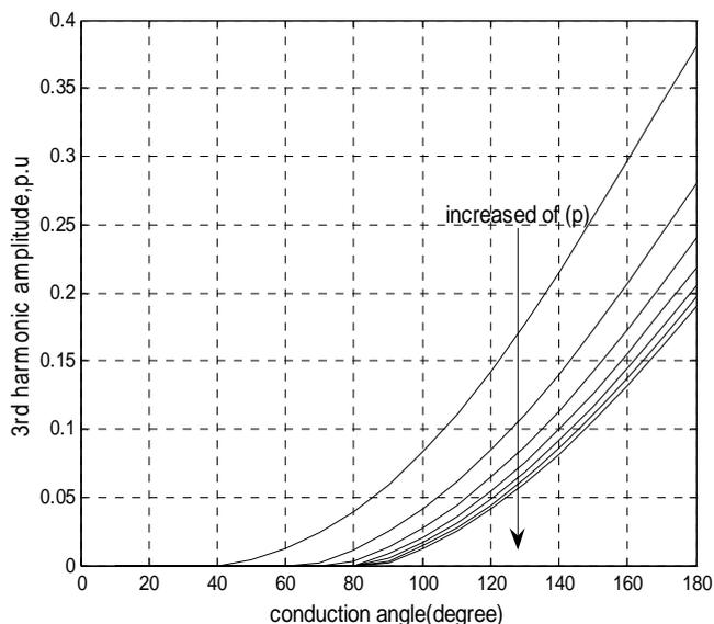
Figure.6 Small-boundary pulse-width technique for  $p=3, 5, 7, \dots, 15$
