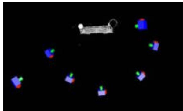
Figure 4. Camera Stations to produce a 3D Model for the left Gate of the stage of Jerash Southern Theatre
