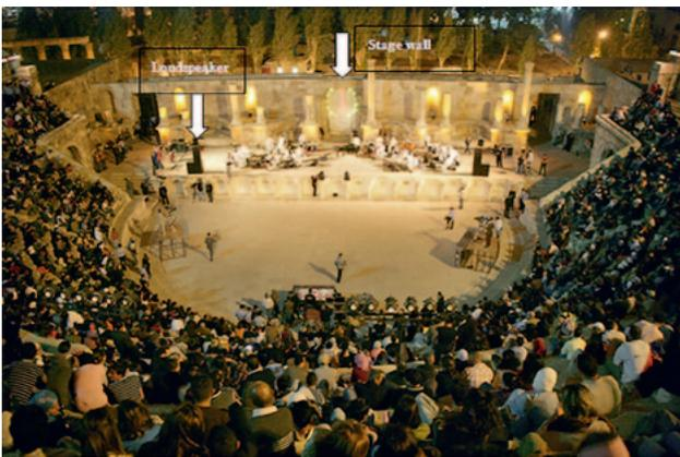
Fig. 3 Philadelphia (Amman) great theatre is used today for performances. The stage wall has been partially restored, but not to its original height. Loudspeakers are placed on the stage but should be located in the orchestra to avoid problems with echoes. Photo: Naif Haddad.
