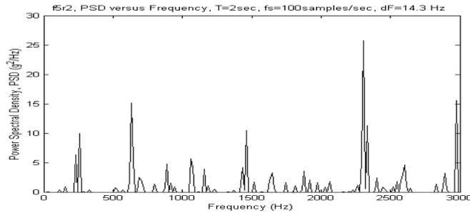
**Fig.1** A sample of power spectrum of the vibration time signal picked up from the crystallizer agitator component
