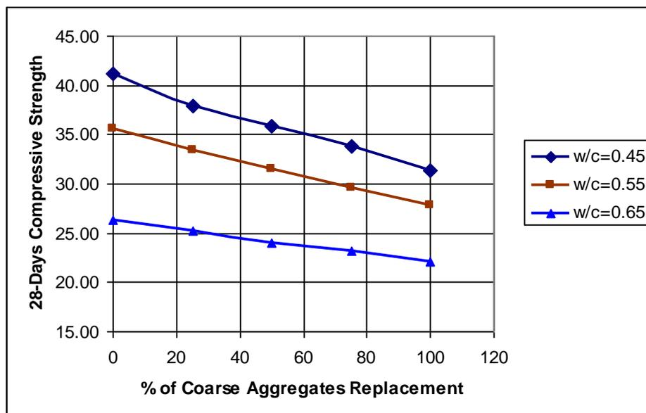
Fig. 3: Relationship between the percentage of the coarse aggregate replaced by concrete rubbles and the 28-day compressive strength.
