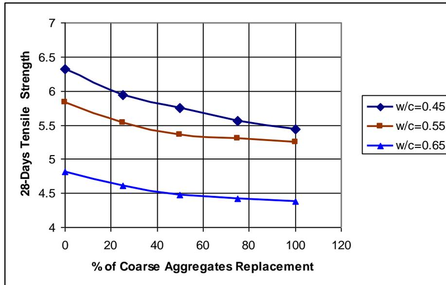
Fig. 4: Relationship between the percentage of the coarse aggregate replaced by concrete rubbles and the 28-day tensile strength
