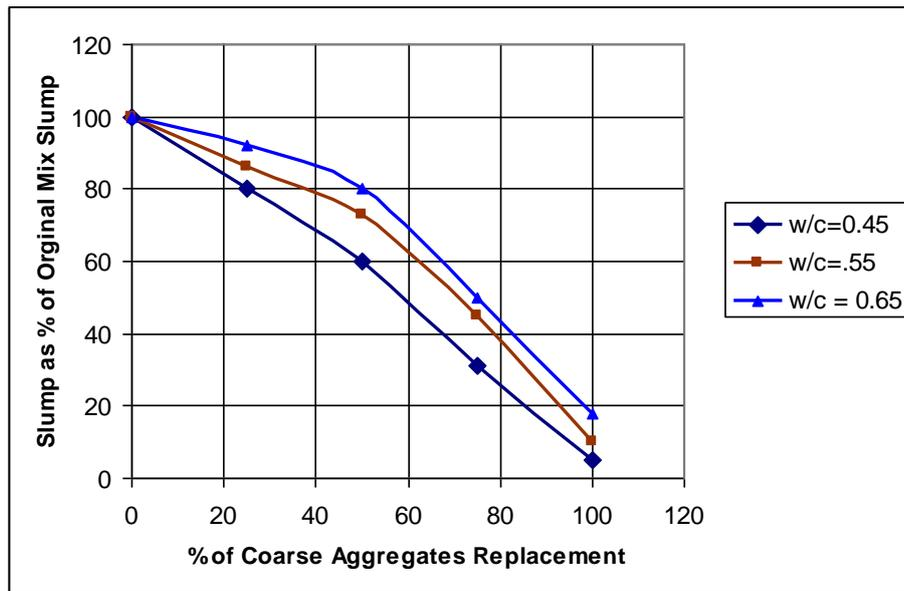
Fig. 2: Relationship between the percentage of the coarse aggregate replaced by concrete rubbles and the percentage of the original slump
