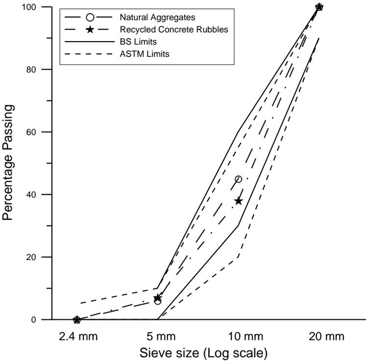
Fig. 1: Grading of both normal aggregate and concrete rubbles
