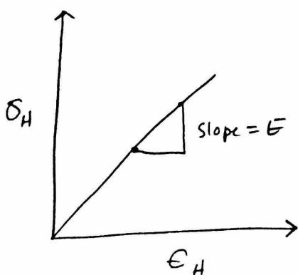
② Open end cylinder  $\rightarrow$  apply  $P \rightarrow$  calculate  $\sigma_H = \frac{Pr}{t}$
