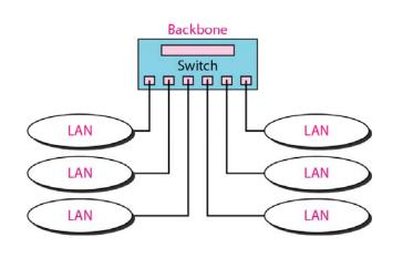
Figure 15.14 Connecting remote LANs with bridges
