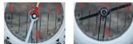
Figure 2.6 How to use the Silva - type compass - clinometer to measure the orientation and dip of a plane using the contact method. The parts of the compass - clinometer are shown in Figure 2.3 d and e.
