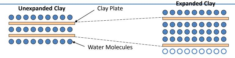
**Expansion** resulting from increased water content can drastically **reduce the shear strength** of an Earth material, often contributing to downslope movement.
