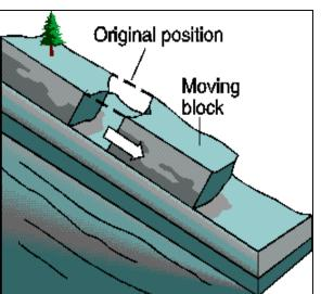
**Slides** involve the rapid displacement of masses of rock or sediment in one direction (translational), with no rotation.
