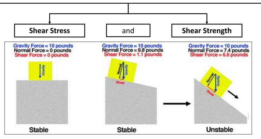
**Shear stress** causes movement of the body parallel to the slope.
