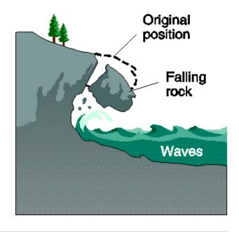
Water can act in other ways that contribute to slope instability, such as undercutting the base of the slope or altering the chemical composition of the sediment.
