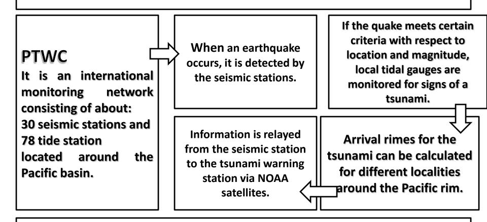
The minimum time required to gather this information and issue a warning is 1 hour; since tsunamis typically travel at 750 km/h, this means that the Pacific-wide early-warning system is effective only for communities located more than 750 km from the epicenter.
