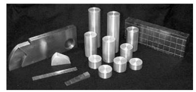
signal. By comparing the signal from the reference standard to that received from the actual flaw, the inspector can estimate the flaw size.
