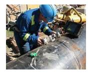
In general, ultrasonic testing is based on the capture and quantification of either the reflected waves (*pulse-echo*) or the transmitted waves (*through-transmission*). Each of the two types is used in certain applications, but generally, pulse echo systems
