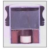
The <u>thickness of the active element</u> is determined by the desired frequency of the transducer. A thin wafer element <u>vibrates with a wavelength that is twice its thickness</u>. Therefore, piezoelectric crystals are cut to a thickness that is 1/2 the desired radiated wavelength. The higher the frequency of the transducer, the thinner the active element is.
