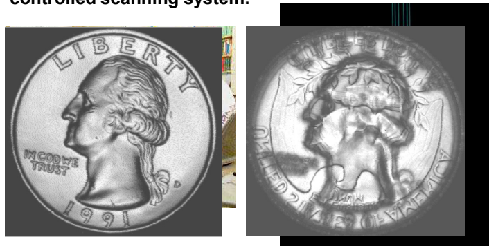
Gray scale image produced using the sound reflected from the front surface of the coin
