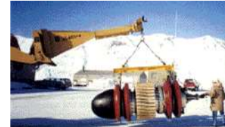
Magnetic flux leakage inspection. This device, known as a pig, is placed in the pipeline and collects data on the condition of the pipe as it is pushed along by whatever is being transported.
