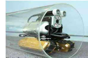
Photo Courtesy of Inuktun Remote visual inspection using a robotic crawler.
